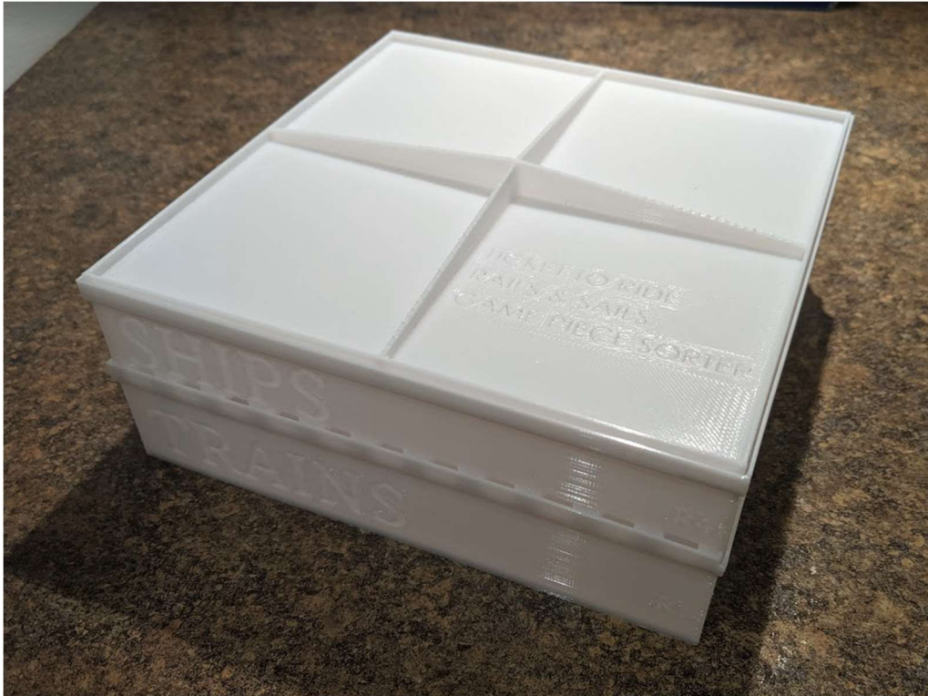
Figure 6. Printed prototype of stacked shaker design, assembled
