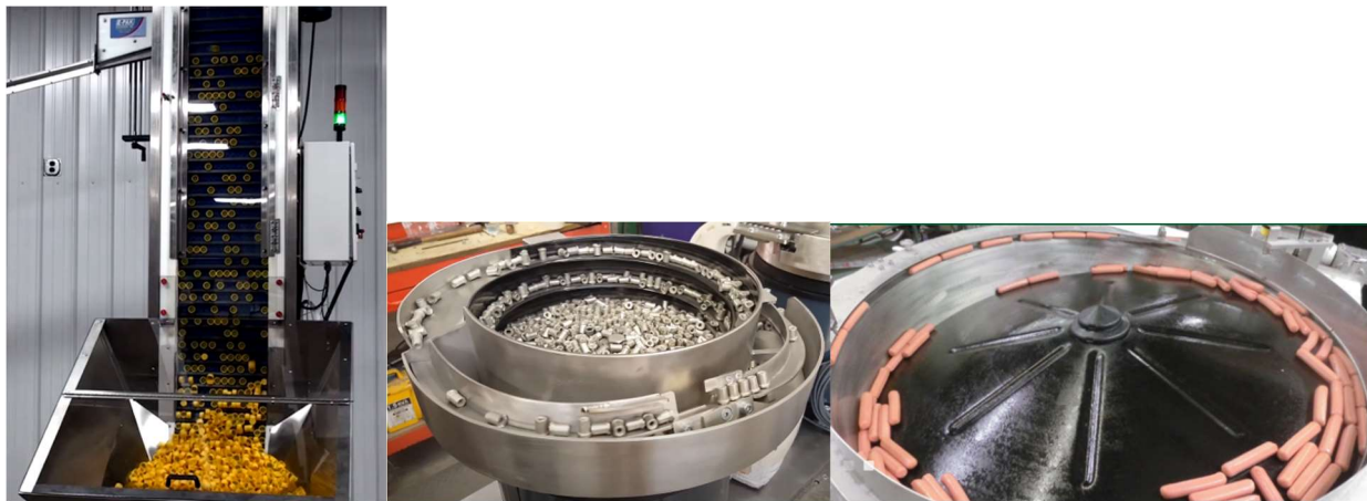
Figure 2. A) Elevator feeder [2], B) Vibratory bowl feeder [3], C) Centrifugal feeder [4]
