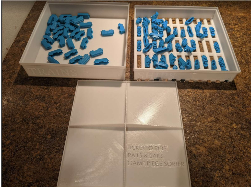
Figure 7. Printed prototype of stacked shaker design, disassembled
